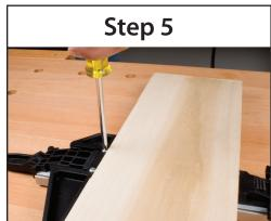
With the clamp and the stock locked into position, secure the 90° Head to the clamp with the two self-tapping screws provided.
