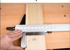
Select a piece of stock that you know is square. Place the selected stock in between the clamp jaws with the 90° head in place. Slide the adjustable clamp head against the side of the stock. Check to make sure the stock is at 90° with a square. (Do not lock clamp until you are finished squaring the 90° Head)
