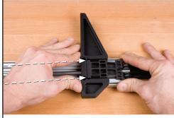
Slide the 90° Head firmly up against the fixed jaw pad, making sure the 90° Head does not have any side to side movement. Step 3
