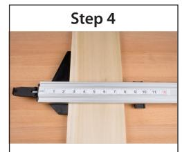
Once the clamp is at 90° to the board, lock the clamp to the stock piece with the cam lock lever.
