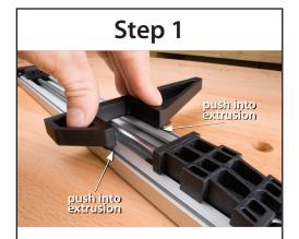
Push the grooved ends of the 90° Head into the under side extrusions of the PRO-Grip<sup>™</sup> Clamp. The 90° Head should fit snug in the extrusion. Step 2
